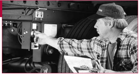
QUIK-DRAW allows drivers to disengage the slider's lock pins using only fingertip effort.
